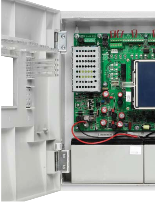
DF6100 control panel, interior
